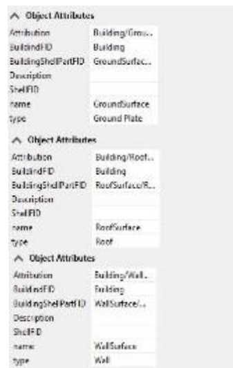
Figure 12: The attributes rendered to the ground, the roof and the wall surfaces
